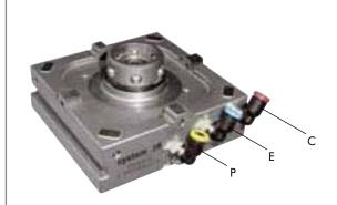
Clamping mechanically with pneumatic release provides maximum operational safety and reliability.
