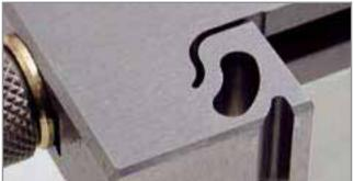
The unique, patented asymmetric design of the locking jaws gives extremely high locking force and enhances the contact between the workpiece and the reference surface at the same time.
